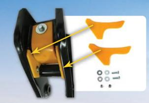
Pictured: Reyco 86AR Hanger installed with EWP Warepad and Hanger Side Plates. Pictured to the right of the Hangers is a sample of a Hanger Side Plate Kit.
