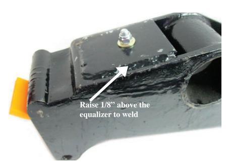
DO: Install the EWP Warepad into a 21B Open Top Equalizer. You can install the EWP Equalizer Warepad into a 21B Open Top Equalizer. First, you must weld in a 1/4"steel plate. The plate should be raised 1/8" above the equalizer so that you get a strong weld.
