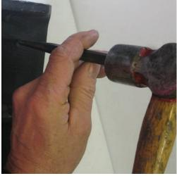
OR: Mark the location of the hole using a center punch to create a small dent in the steel. The dent marks the location and helps keep the drill bit from slicing across the steel. Hold the center punch in position and strike it with a hammer to make your mark.
