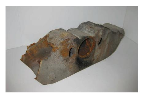
DON'T: Install EWP Warepads into a compromised hanger or equalizer. We do not recommend installing EWP into a worn out OEM part. The Warepads are designed to save on additional wear to the hanger, equalizer and leaf spring. They are not designed to improve a part that is not salvageable.
