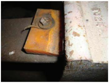
DON'T: Don't attach the EWP Equalizer Warepad on the end of the spring. The Equalizer Warepad must be attached to the OEM Equalizer.
