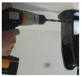
**DO: Drill a pilot hole into OEM Equalizer or OEM Hanger.** Select a drill bit that is 50 percent smaller than the size of the finished hole for a pilot bit. For instance:
