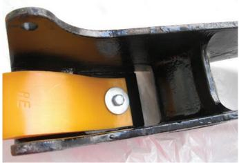
DO: Place the washer directly on the EWP Warepad. For all bolt installations, the washer should always be directly on the EWP Warepad. This will prevent the bolt or nut from sliding through the poly pad and causing the pad to fall out.
