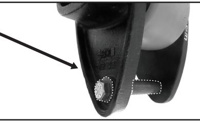
Step 2: Use the Hanger Rebound Hole as a guide to mark the Side Plate. Insert the Side Plate as shown into the Hanger. Hold in place. Mark the Side Plate with a marking pen through the Hanger rebound bolt hole.
